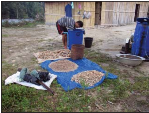
Stones of multiple sizes are gathered and prepared for use in a water filter
